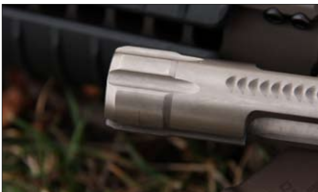
Intelligent enhancements: All LWRCI carriers have been increased in diameter at the rear to deal with carrier tilt (left). The thrust lug on the carrier is pressed and locked into a hefty dovetail (right).
