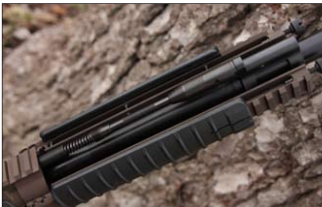
The gas system on the A2 is entirely under the handguard and yet is easily accessible for cleaning.
