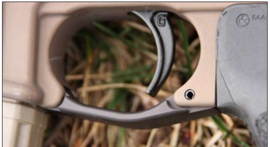
The triggerguard is sculpted and makes shooting with gloves a lot easier.
